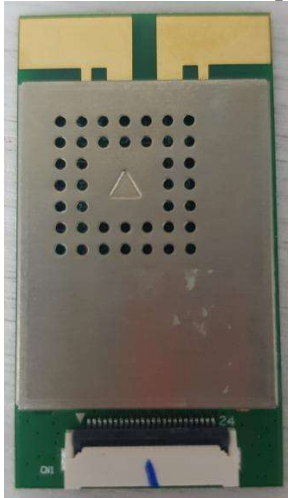
Fig 5.1 5G_MODULE_FPC Module TX with shielding case TX Button View Top View
