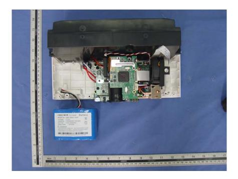
Note: BK01DW45AW, BK01DW45AK, BK01DW45AG, BK01DW45AS, BK01DW45AR "W" is White; "K" is Black; "G" is Gray; "S" is Sliver; "R" is Red, They represent different colors. BK01DW45A\* series' EUT only equipped with a battery. The battery capacity is 13000mAH. The other circuits are all the same.
