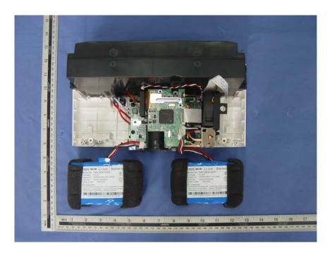
Note: BK02DW45AW, BK02DW45AK, BK02DW45AG, BK02DW45AS, BK02DW45AR "W" is White; "K" is Black; "G" is Gray; "S" is Sliver; "R" is Red, They represent different colors. BK02DW45A\* series' EUT are equipped with two battery. The battery capacity is 15600mAH and 10400mAH respectively. The other circuits are all the same.
