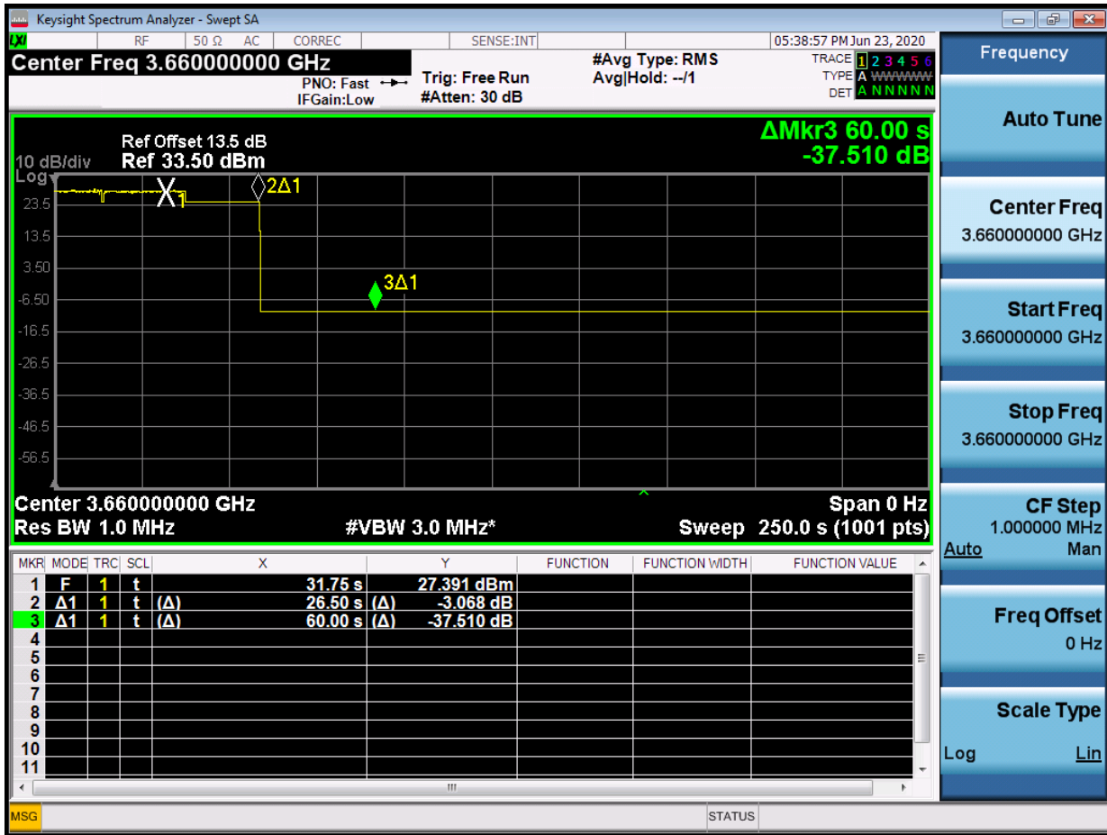
Plot 20. Conducted Measurement - RF transmission stops within 60s. The SAS message is indicated by Marker 1 (X) (WINNF.FT.D.DRG.2)
