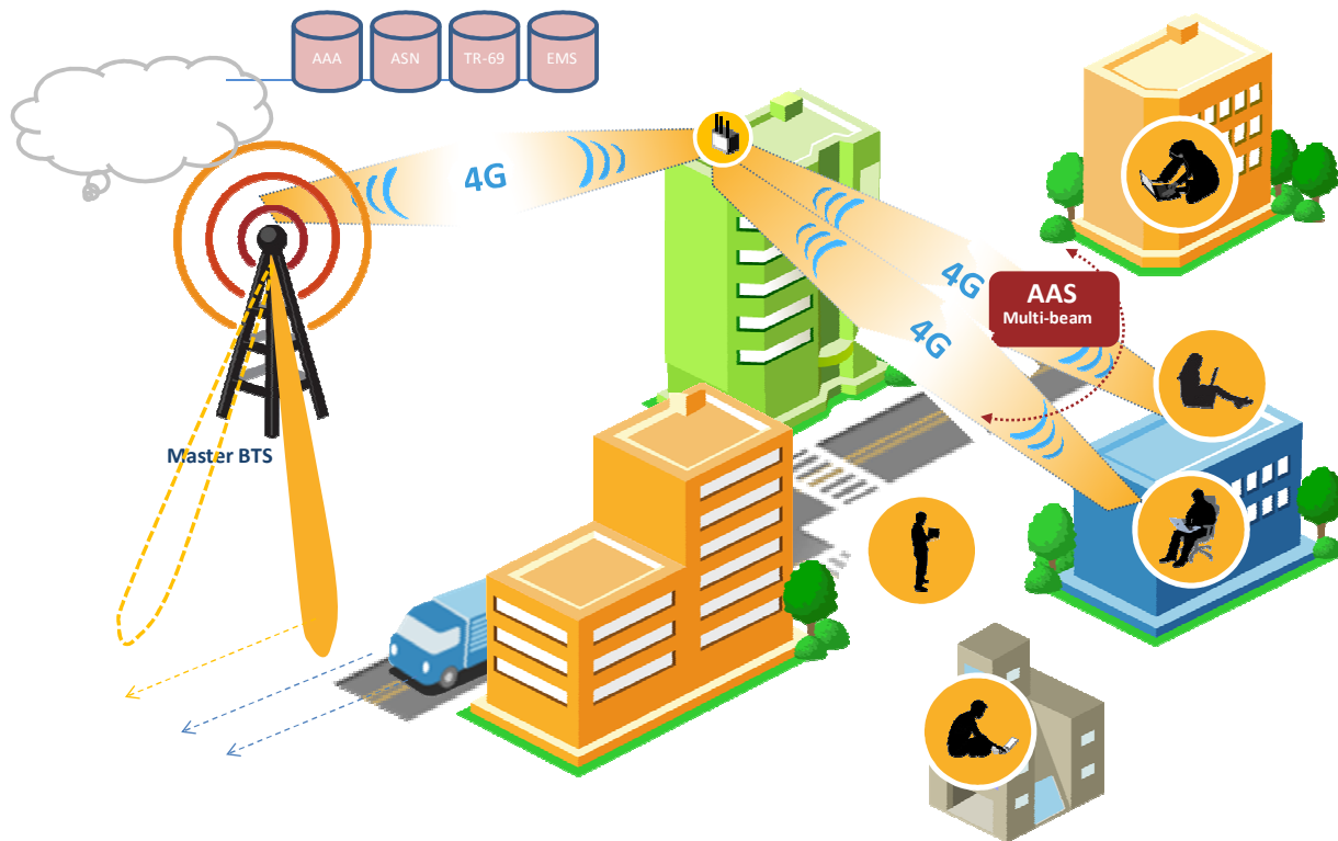
Figure 7 - 802.16e system implementation
