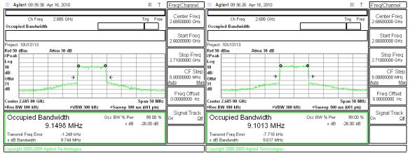
2.5 GHz Fixed Wireless Transceiver FCC ID: XN3-QUANTUM6625
