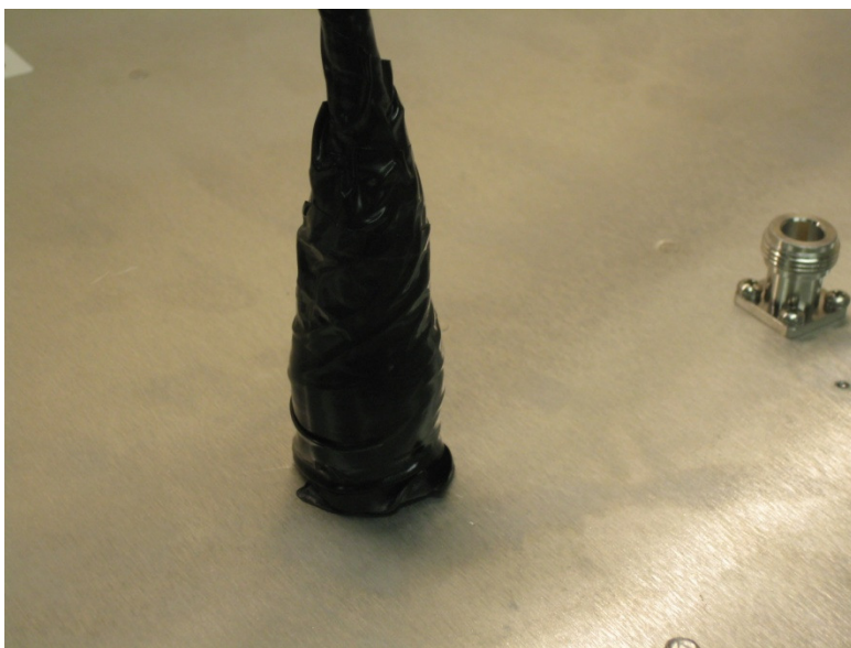
Figure 54- Second Plastic Tape Applied
