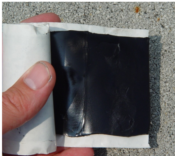
Figure 49 - Butyl Tape Weather Protection
