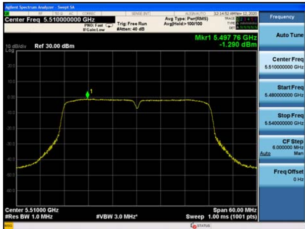
U-NII-2C, 802.11n HT40 Carrier frequency (MHz): 5670
