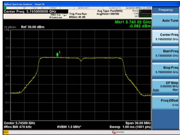
U-NII-3, 802.11n HT20 Carrier frequency (MHz): 5785
