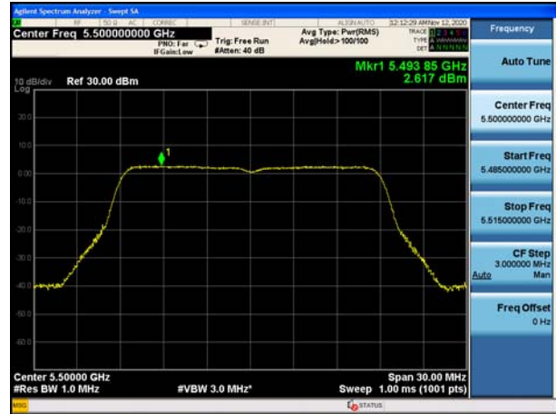
U-NII-2C, 802.11n HT20 Carrier frequency (MHz): 5600
