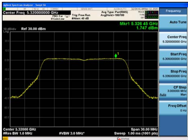
U-NII-2A, 802.11a Carrier frequency (MHz): 5320
