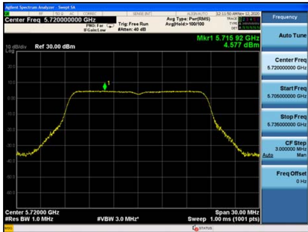
U-NII-2C, 802.11n HT40 Carrier frequency (MHz): 5510
