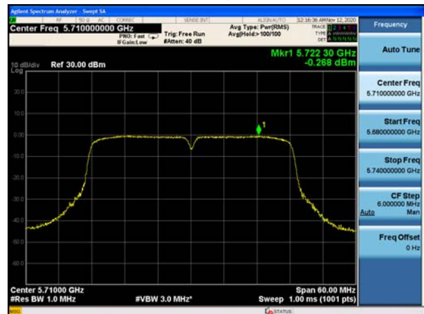
U-NII-2C, 802.11n HT40 Carrier frequency (MHz): 5710
