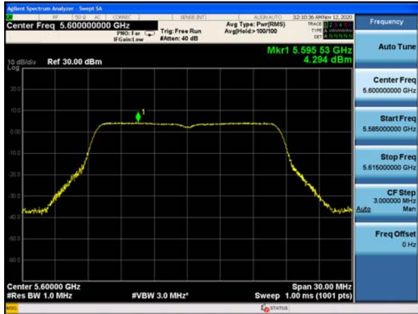
U-NII-2C, 802.11a Carrier frequency (MHz): 5700
