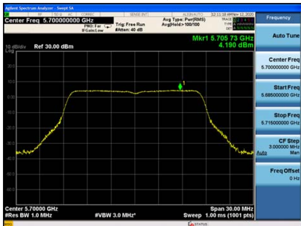
U-NII-2C, 802.11a Carrier frequency (MHz): 5700
