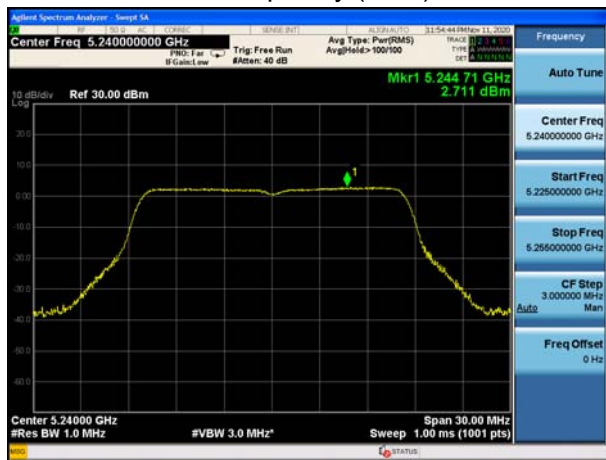
U-NII-1, 802.11a Carrier frequency (MHz):5240
