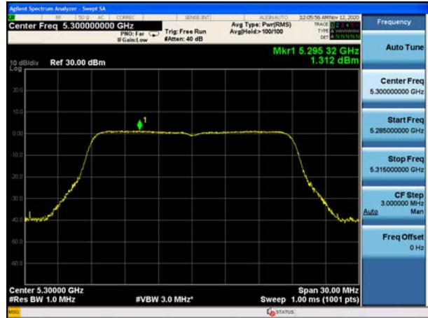
U-NII-2A, 802.11n HT20 Carrier frequency (MHz): 5320
