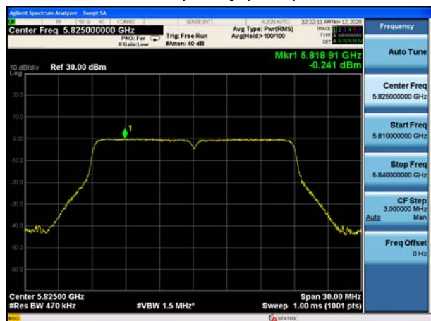
U-NII-3, 802.11n HT20 Carrier frequency (MHz): 5825
