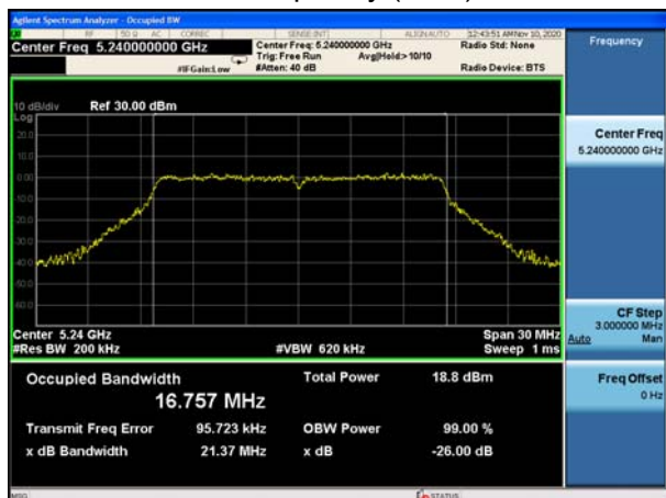
U-NII-1, 802.11a Carrier frequency (MHz):5240
