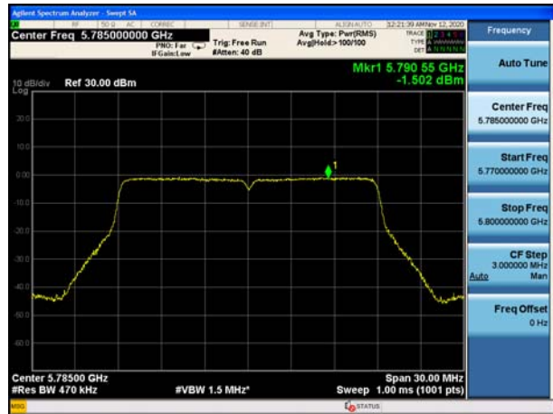
U-NII-3, 802.11n HT20 Carrier frequency (MHz): 5825
