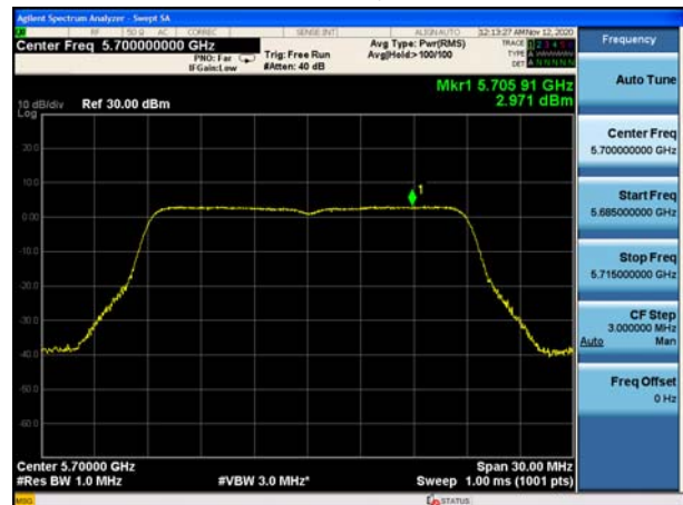
U-NII-2C, 802.11n HT20 Carrier frequency (MHz): 5700
