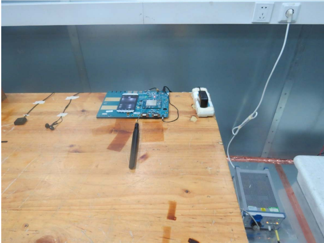
Picture 2 Conducted Emission Test Setup
