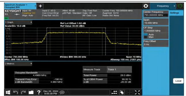
Band14-5MHz-16QAM-23330-25RB#0-PASS
