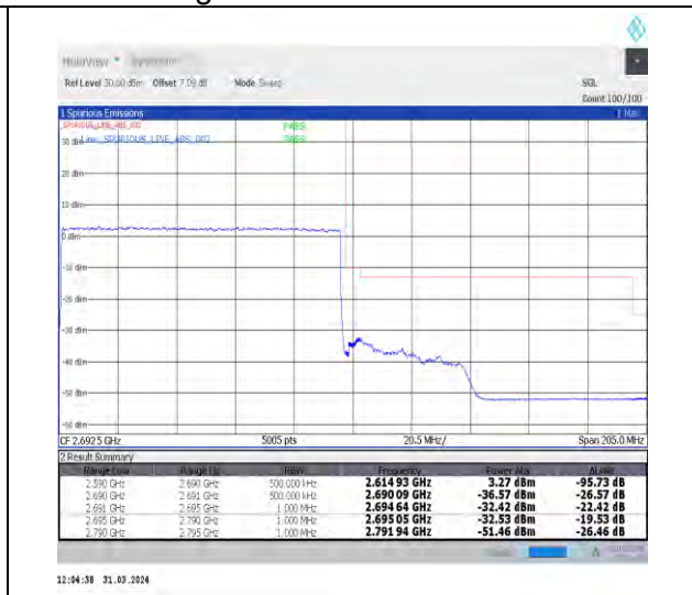
1-N41-30-100-H-3-DFT-PI2BPSK-Outer_Full-270 @0-Ant1-1--PASS-see graph
