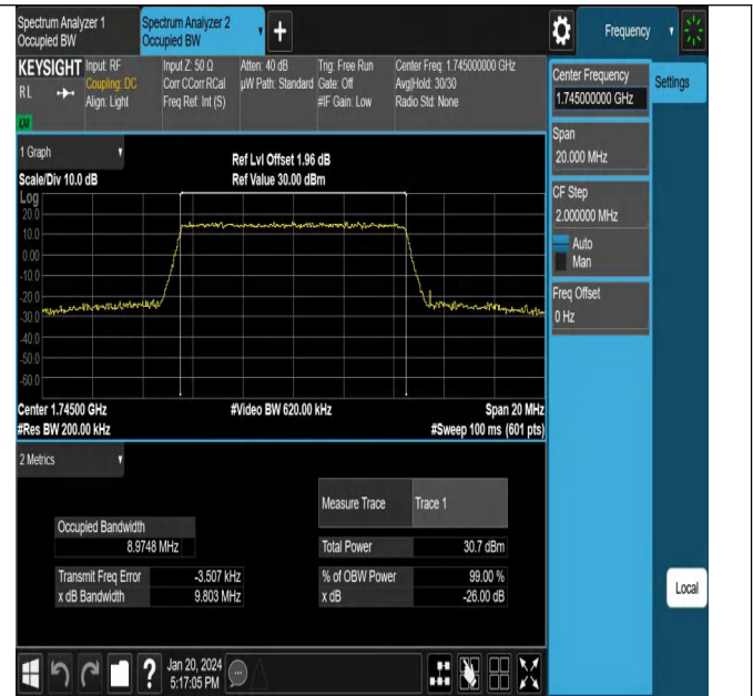
Band66-10MHz-QPSK-132322-50RB#0-PASS
