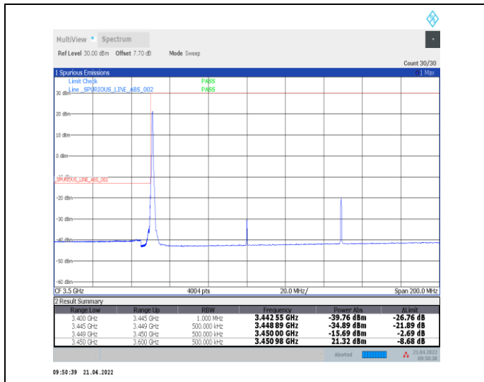
1-N78-3450-3550--30-100-L-1-DFT-PI2BPSK-Edge_1 RB_Left-1@0-Ant0-PASS-see graph
