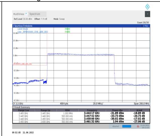
1-N78-3450-3550--30-100-L-3-DFT-PI2BPSK-Out er_Full-270@0-Ant0-PASS-see graph
