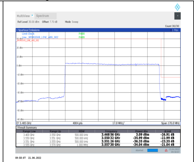
1-N78-3450-3550--30-100-H-3-DFT-PI2BPSK-Out er_Full-270@0-Ant0-PASS-see graph
