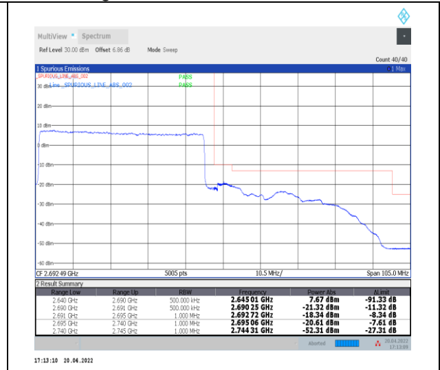
1-N41--30-50-H-3-DFT-PI2BPSK-Outer_Full-128 @0-Ant0-PASS-see graph
