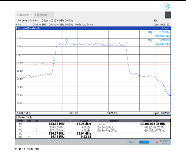
1-N5--15-15-H-4-DFT-64QAM-Outer_Full-75@0-Ant-0 0-13.406-14.490≤15-PASS
