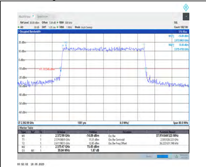
1-N41-PC1-30-40-M-7-CP-16QAM-Outer_Full-106@0 0-Ant1-37.915-39.840-≤40-PASS
