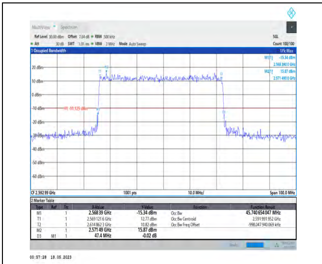
1-N41-PC1-30-50-M-3-DFT-16QAM-Outer_Full-128 @0-Ant1-45.741-47.400-≤50-PASS
