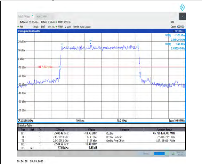
1-N41-PC1-30-50-L-1-DFT-QPSK-Outer_Full-128 @0-Ant1-45.726-47.600-≤50-PASS
