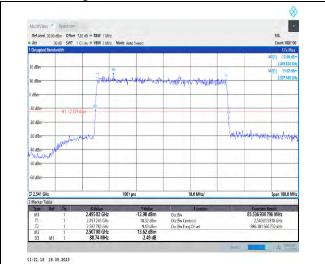
1-N41-PC1-30-90-L-5-DFT-256QAM-Outer_Full-240 @0-Ant1-85.537-88.740-≤90-PASS
