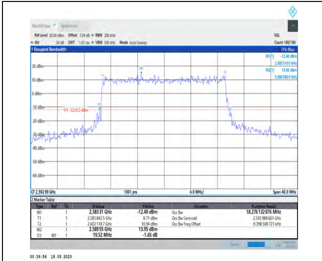
1-N41-PC1-30-20-M-8-CP-64QAM-Outer_Full-51@0 -Ant1-18.276-19.520-≤20-PASS
