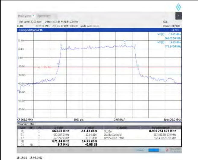
1-N71--15-10-L-1-DFT-QPSK-Outer_Full-50@0-Ant1 -8.933-9.700≤10-PASS
