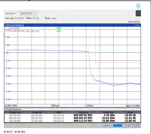
1-N71--15-10-H-3-DFT-PI2BPSK-Outer_Full-50@ 0-Ant1-PASS-see graph
