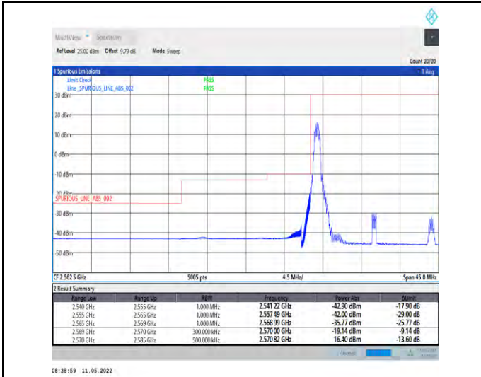
1-N38-PC2-30-15-L-4-CP-QPSK-Edge_1RB_Left-1@0 -Ant1-PASS-see graph
