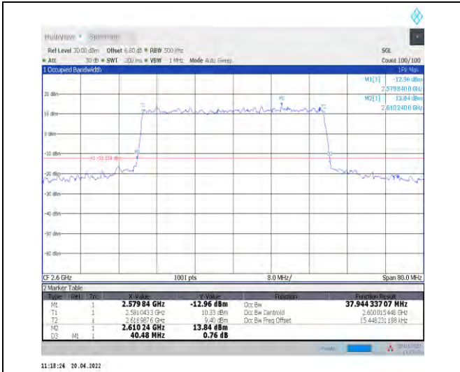
1-N38--30-40-H-7-CP-16QAM-Outer_Full-106@0-An t1-37.944-40.480-≤40-PASS
