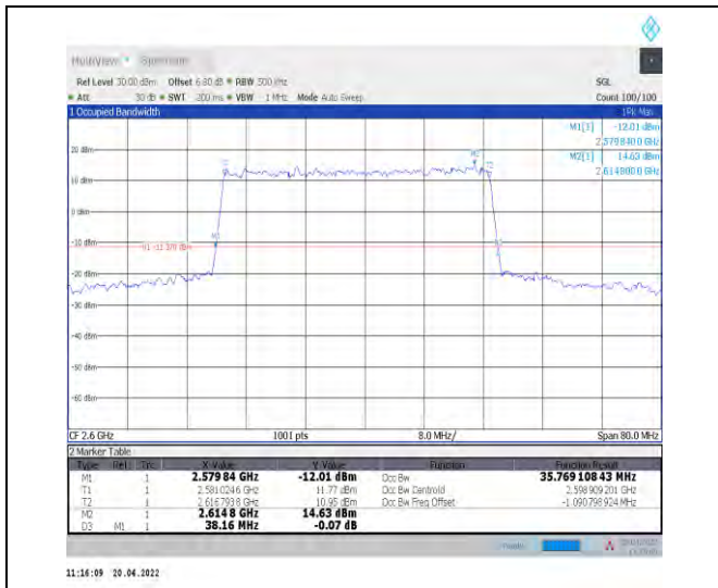
1-N38--30-40-H-3-DFT-16QAM-Outer_Full-100@0-A nt1-35.769-38.160-≤40-PASS
