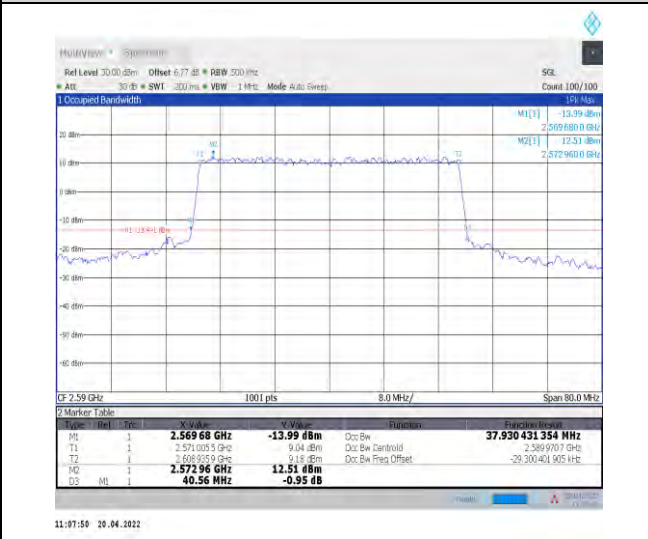
1-N38--30-40-L-8-CP-64QAM-Outer_Full-106@0-Ant t1-37.93-40.560-<=40-PASS
