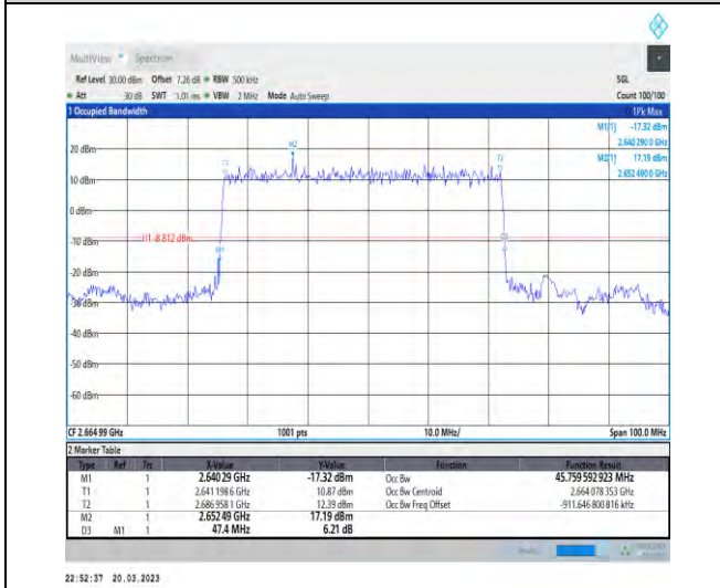
1-N41-30-50-H-2-DFT-PI2BPSK-Outer_Full-128@0-Ant1 Ant1-45.76-47.400-≤50-PASS
