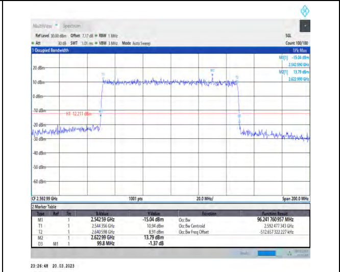
1-N41-30-100-M-4-DFT-64QAM-Outer_Full-270@0-A Ant1-96.242-99.800-≤100-PASS
