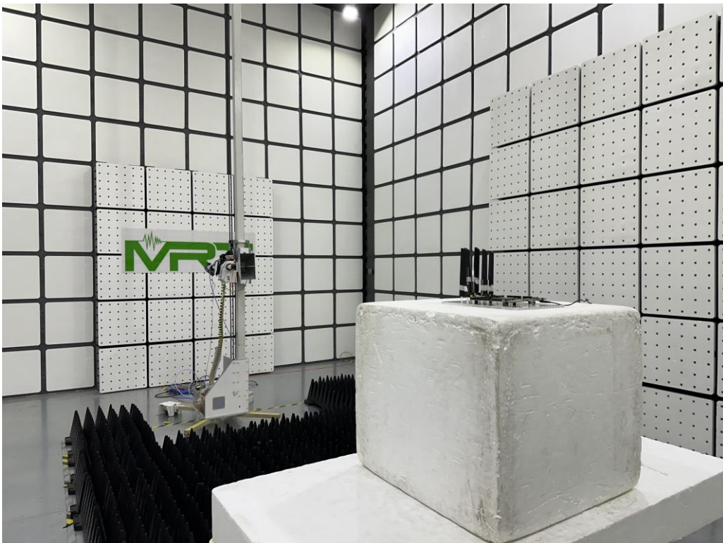
Description: Radiated Spurious Emission Test Setup for 1GHz to 18GHz
