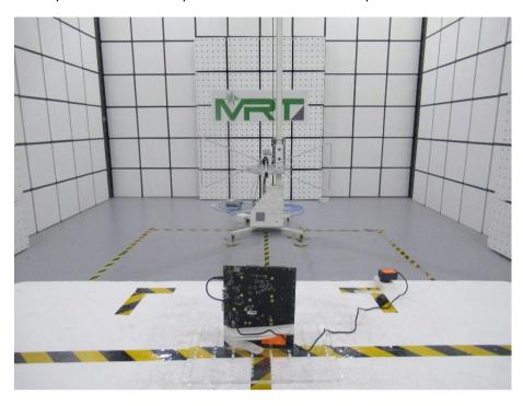
Description: Transmitter Spurious Emissions Test Setup for above 1GHz
