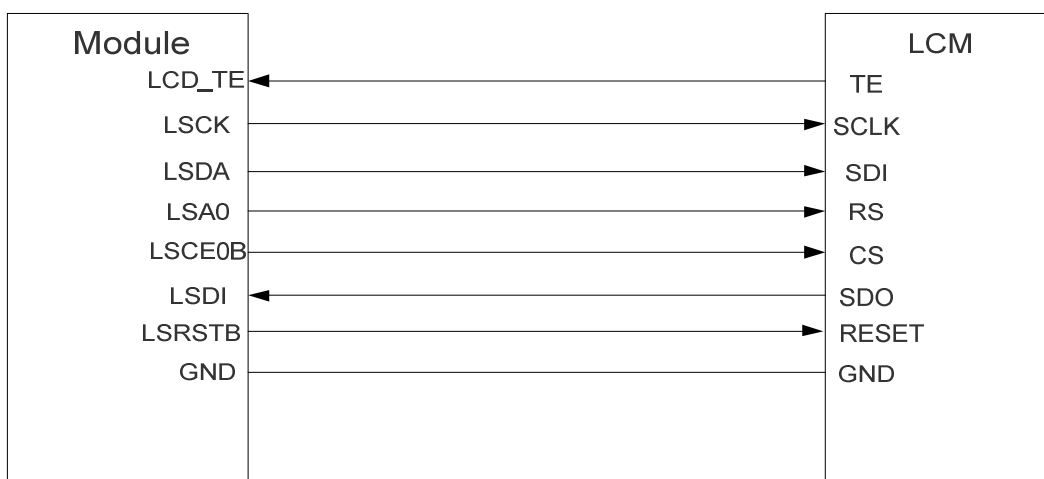
Figure 20: Reference Circuit Design for LCM Interface
