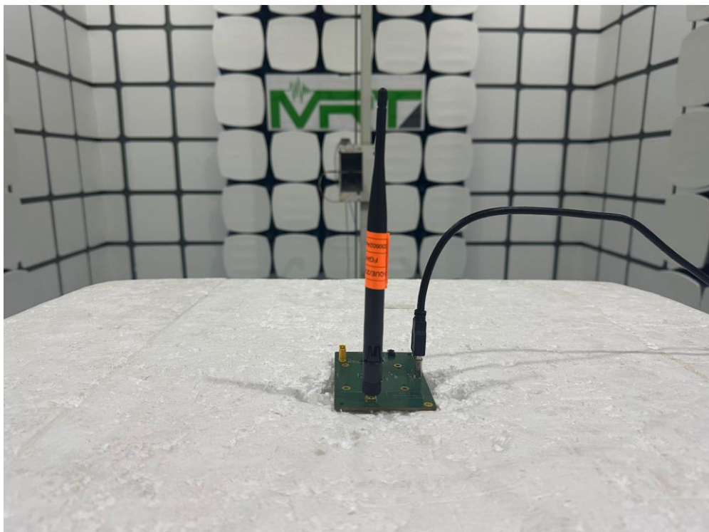
Description: Radiated Spurious Emission Test Setup for Above 1GHz – Z axis
