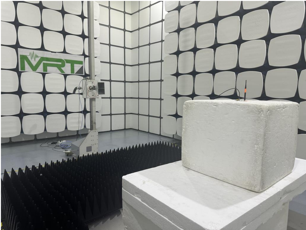
Description: Radiated Spurious Emission Test Setup for Above 1GHz – Z axis
