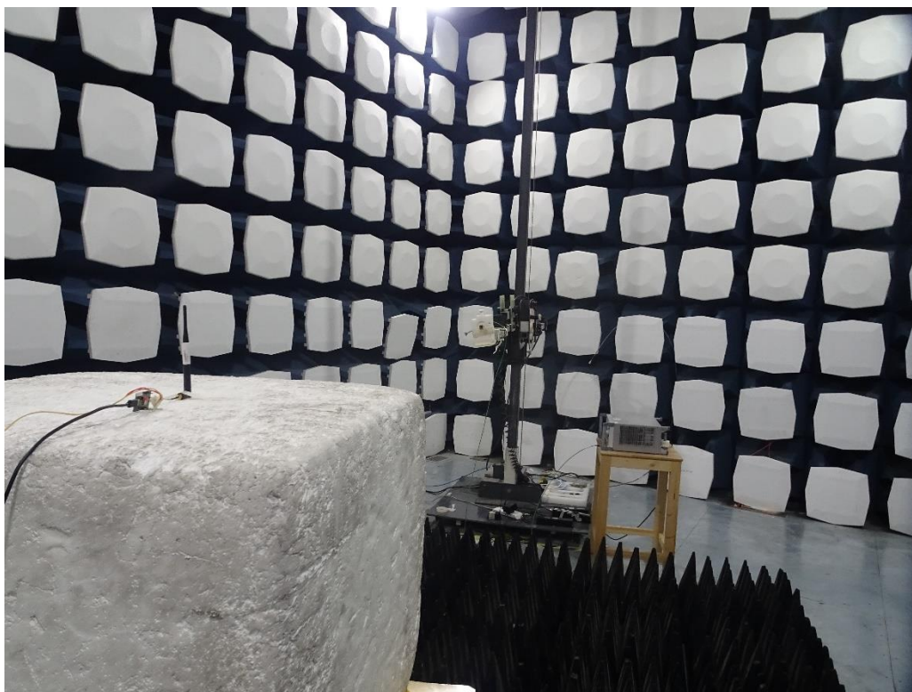
Picture 1 Radiated Emission Test Setup
