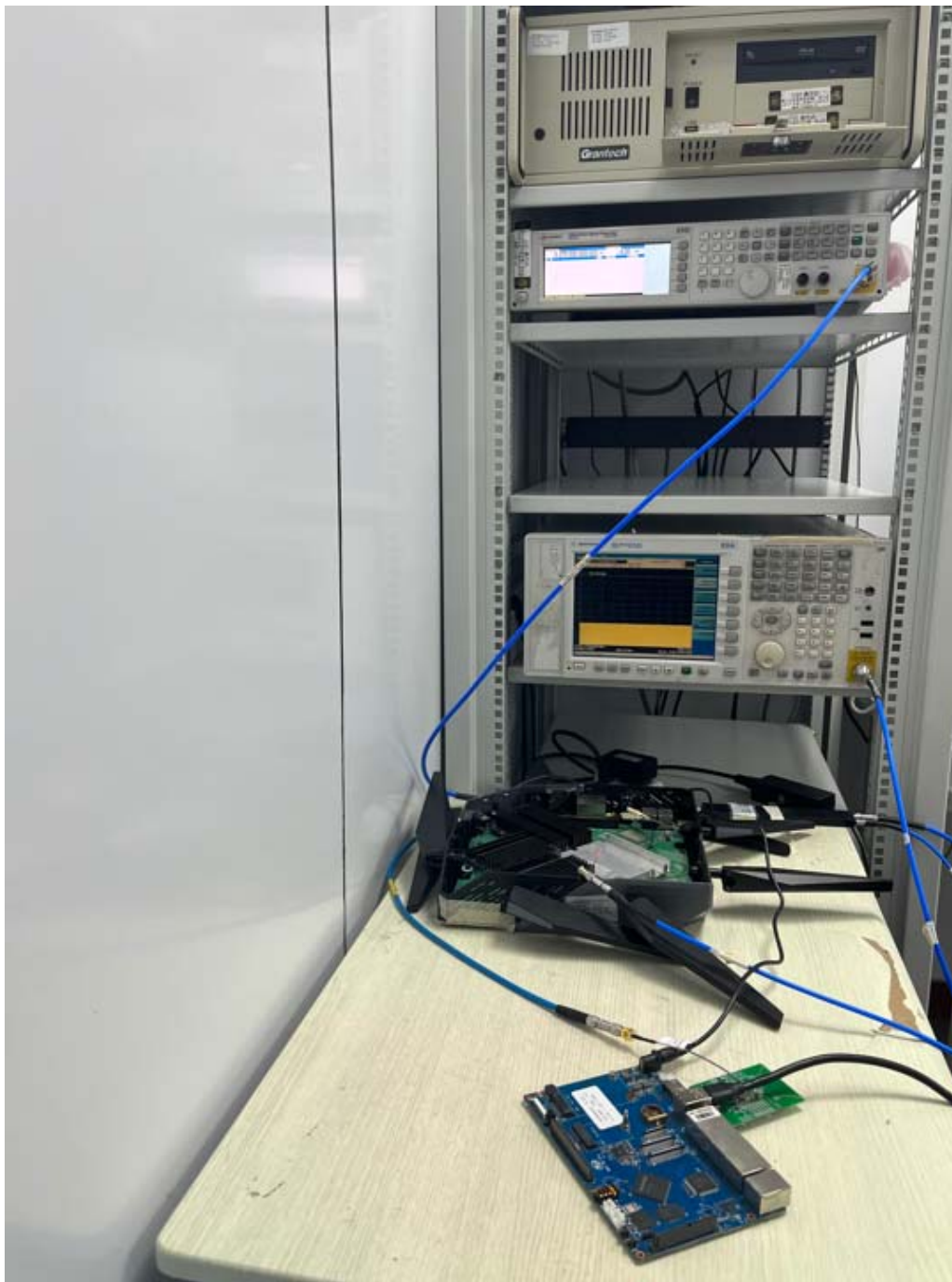
Picture 1 DFS Test Setup
