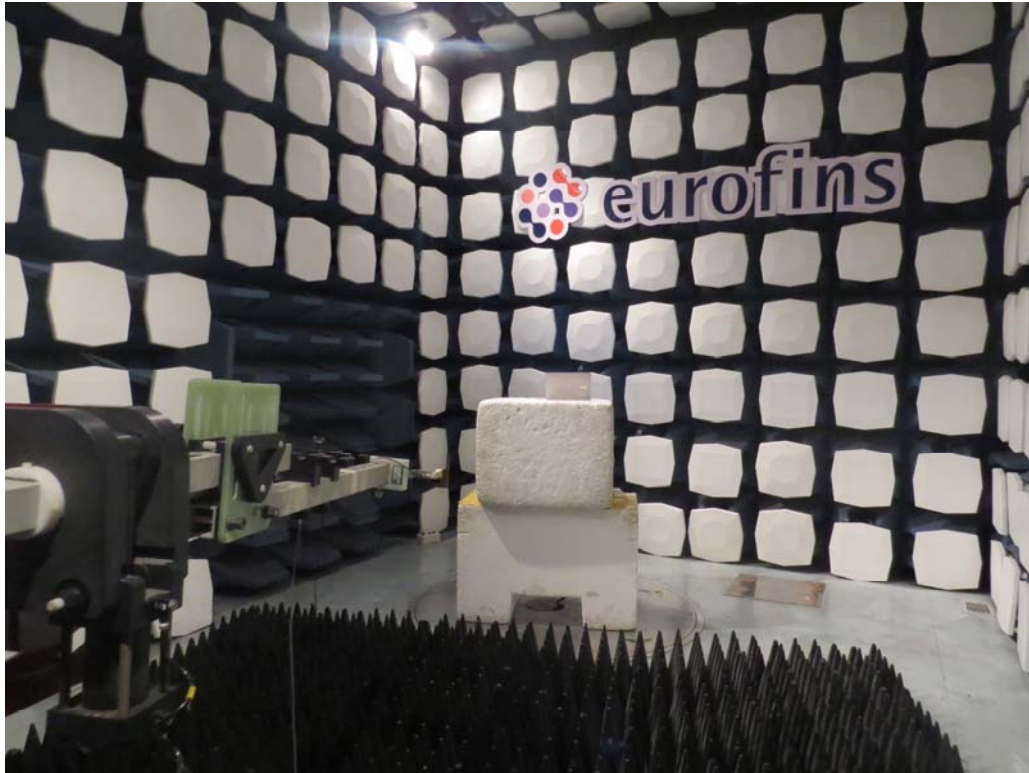
Picture 1 Radiated Emission Test Setup
