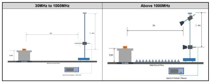
Antenna Tower meets ANSI C63.4 requirements for measurements above 1 GHz by keeping the antenna aimed at the EUT during the antenna's ascent/ descent along the antenna mast.
