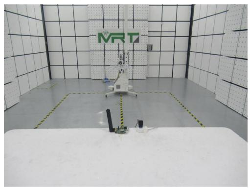
Description: Radiated Spurious Emissions Test Setup for Below 1GHz
