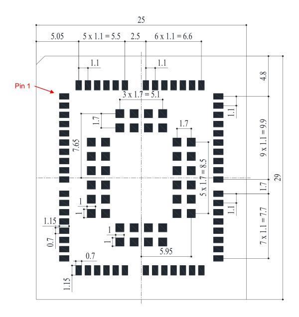
Figure 39: Recommended Footprint (Top View)
