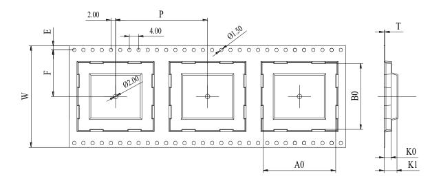
Figure 42: Carrier Tape Dimension Drawing
