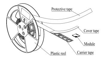
Place the module into the carrier tape and use the cover tape to cover it; then wind the heat-sealed carrier tape to the plastic reel and use the protective tape for protection. 1 plastic reel can load 250 modules.
