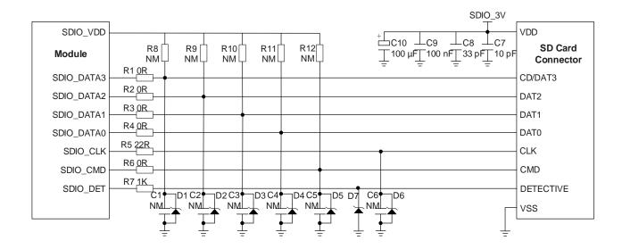
Figure 22: Reference Circuit of SD Card Interface
