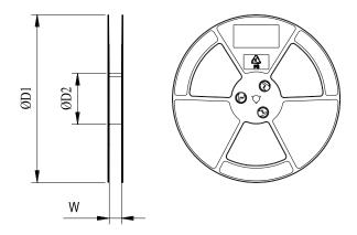
Figure 43: Plastic Reel Dimension Drawing
