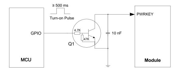
Figure 10: Reference Circuit of Turning On the Module Using Driving Circuit
