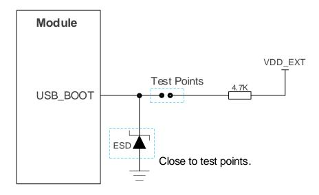
Figure 18: Reference Circuit of USB\_BOOT Interface
