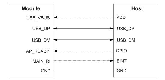
Figure 6: Block Diagram of Application with NAIN\_RI Function in Sleep Mode
