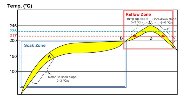
Figure 41: Recommended Reflow Soldering Thermal Profile
