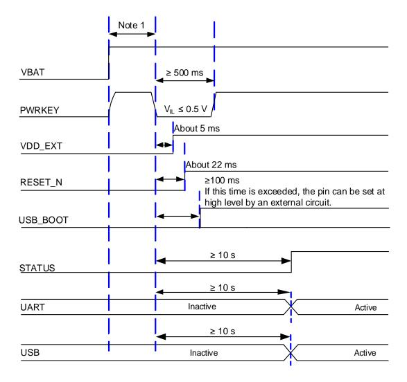
Figure 12: Power-up Timing
