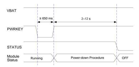
Figure 13: Power-down Timing
