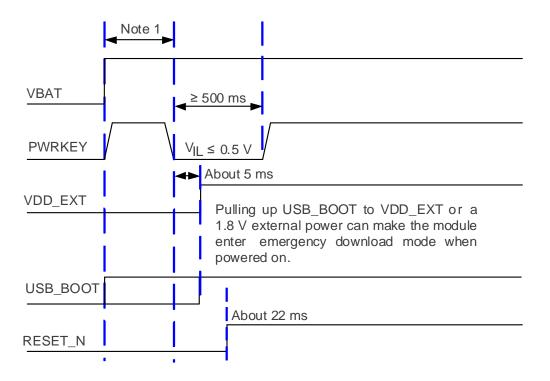
Figure 19: Timing Sequence for Entering Emergency Download Mode
