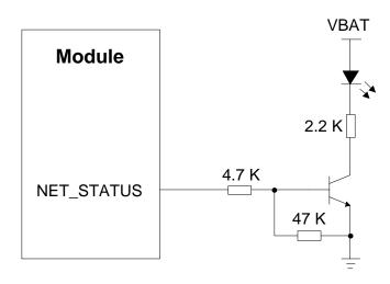
Figure 27: Reference Design of Network Status Indication
