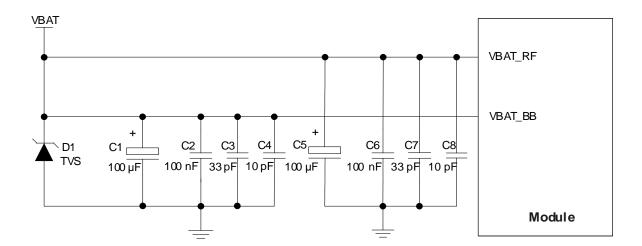
Figure 9: Star Configuration of Power Supply
