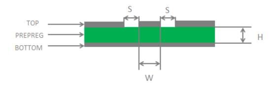
Figure 31: Coplanar Waveguide Design on a 2-layer PCB
