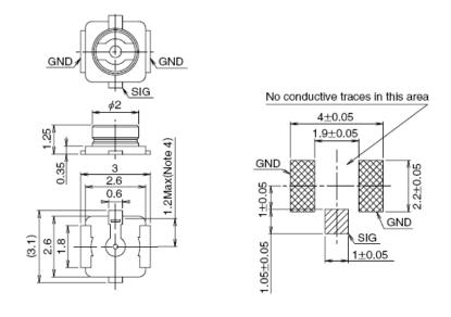
Figure 34: Dimensions of the Receptacle (Unit: mm)
