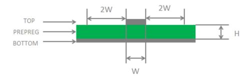
Figure 30: Microstrip Design on a 2-layer PCB
