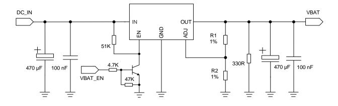
Figure 8: Reference Design of Power Supply
