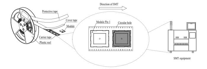
**Figure 44: Mounting Direction**
