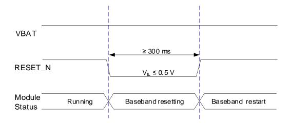
Figure 16: Timing of Reset
