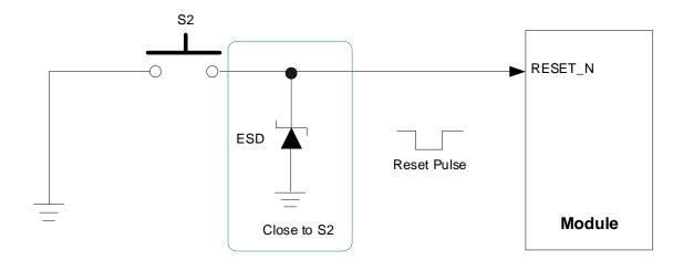
Figure 15: Reference Circuit of RESET\_N with Button
