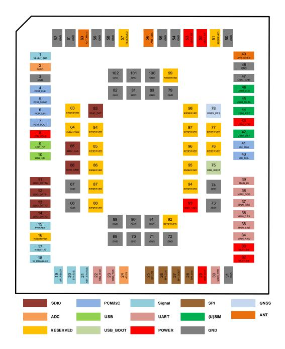
Figure 2: Pin Assignment (Top View)
