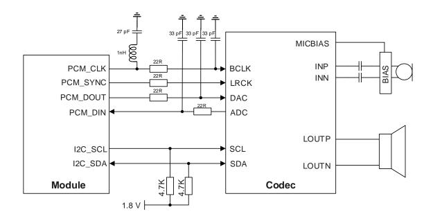
Figure 26: Reference Design of PCM and I2C Interfaces
