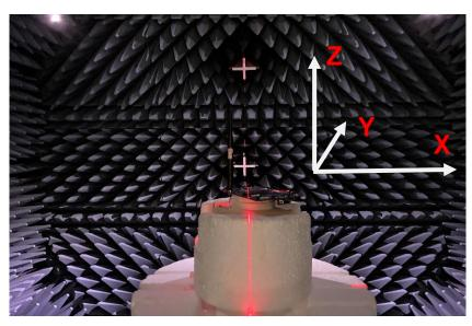
H plane: the tangent of XY E1 plane: the tangent of XZ E2 plane: the tangent of YZ
