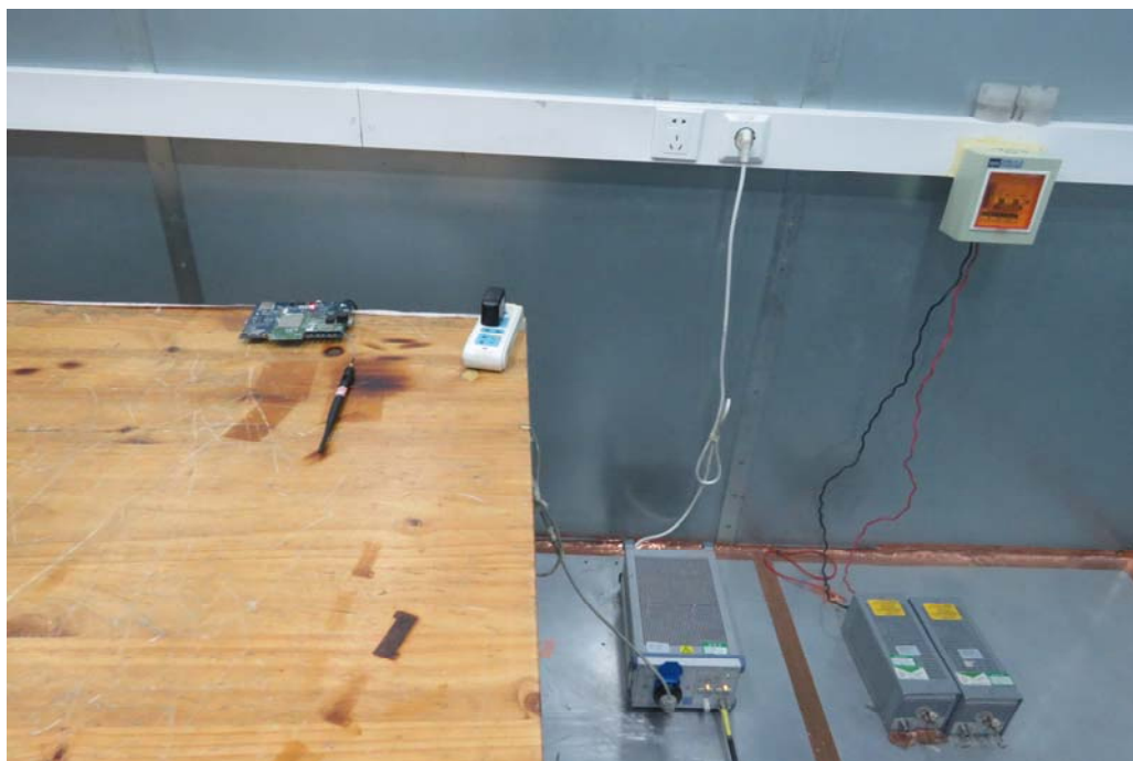
Picture 2 Conducted Emission Test Setup
