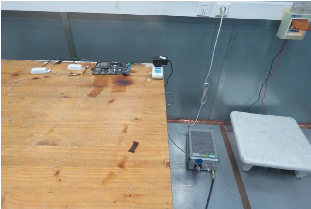
Picture 2 Conducted Emission Test Setup
