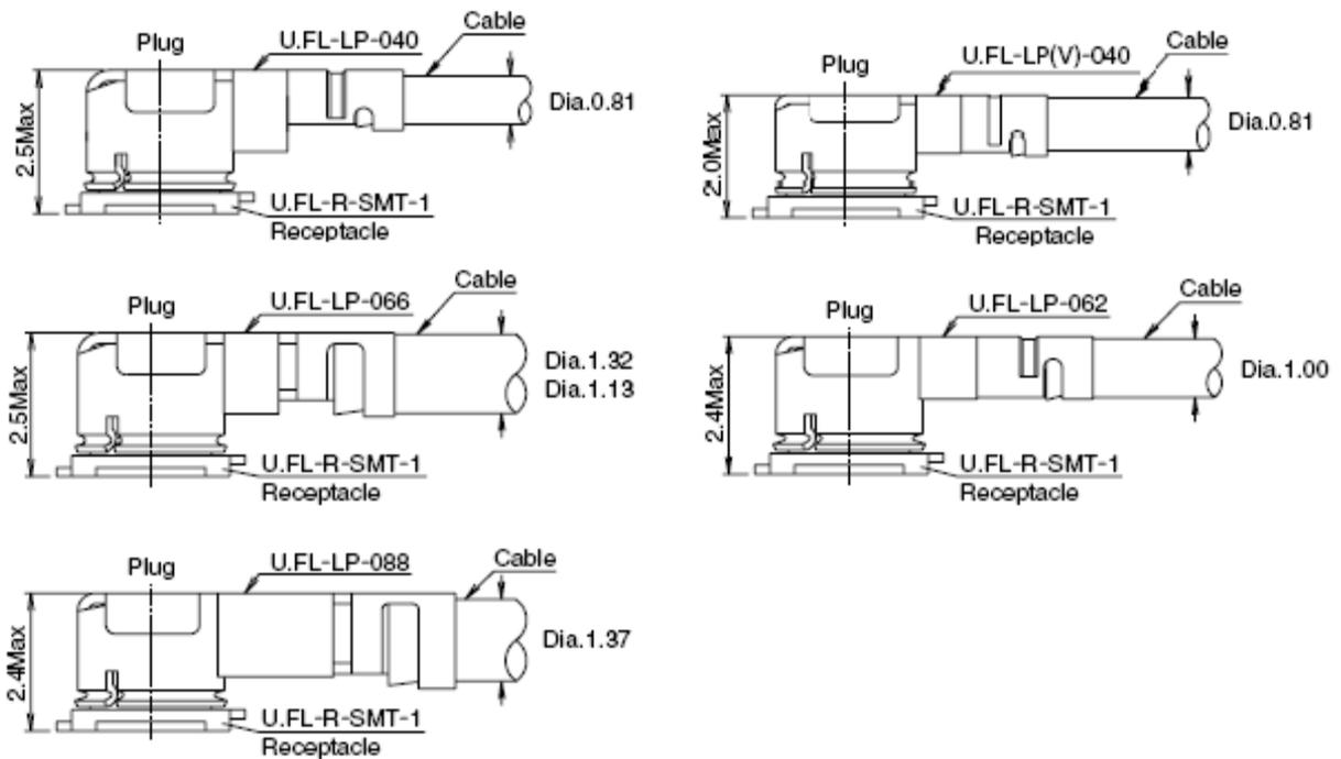
**Figure 35: Space Factor of Mated Connectors (Unit: mm)**
