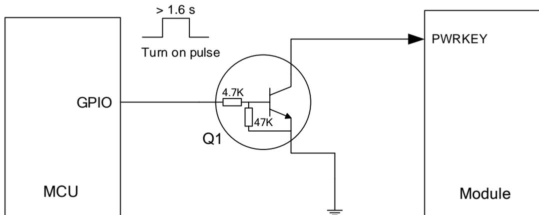
**Figure 7: Turn On the Module Using Driving Circuit**
