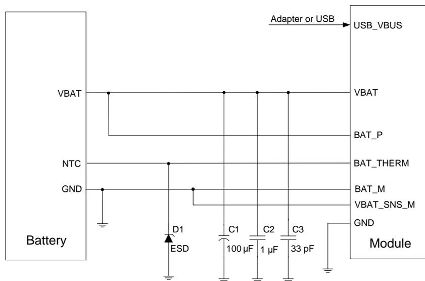
**Figure 3: Reference Design for Battery Charging Circuit**
