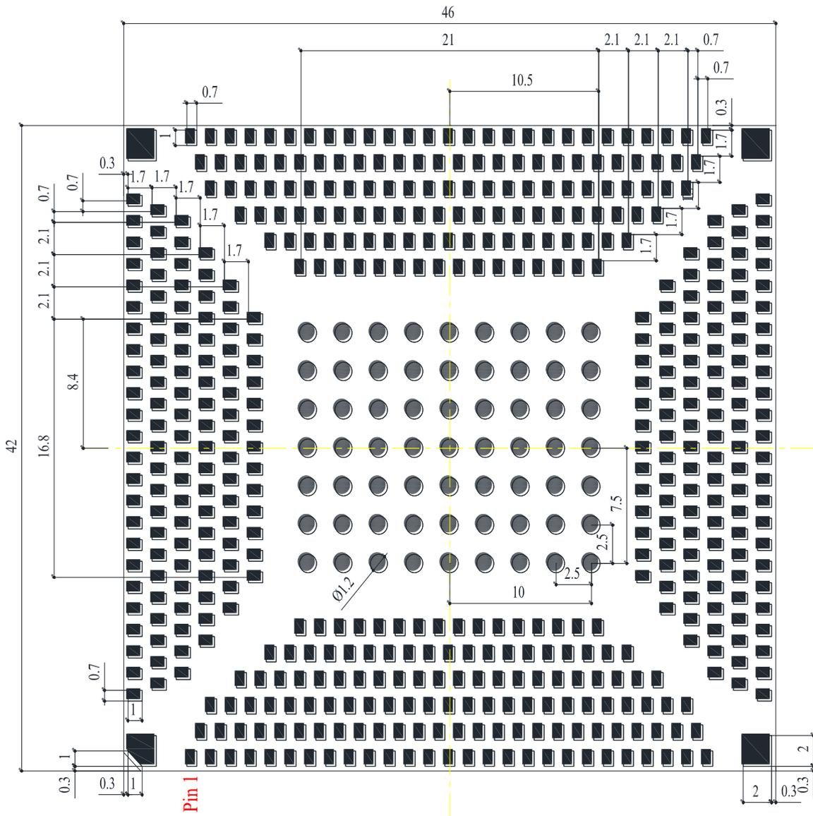
Figure 38: Recommended Footprint (Top View)
