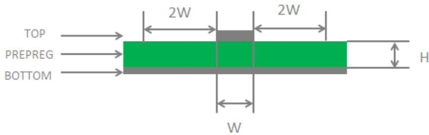
**Figure 29: Microstrip Design on a 2-layer PCB**
