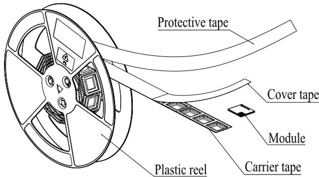
Place the module into the carrier tape and use the cover tape to cover them; then wind the heat-sealed carrier tape to the plastic reel and use the protective tape for protection. One plastic reel can load 200 modules.
