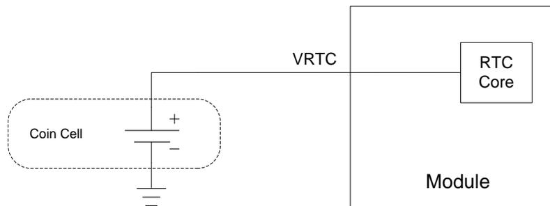
**Figure 12: RTC Powered by a Coin Cell**
