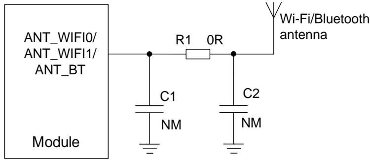
**Figure 28: Reference Design for Wi-Fi/Bluetooth Antenna Interface**
