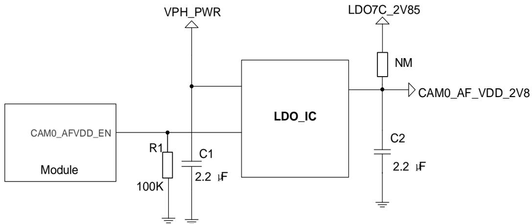
**Figure 25: Reference Design of Camera Power Supply**
