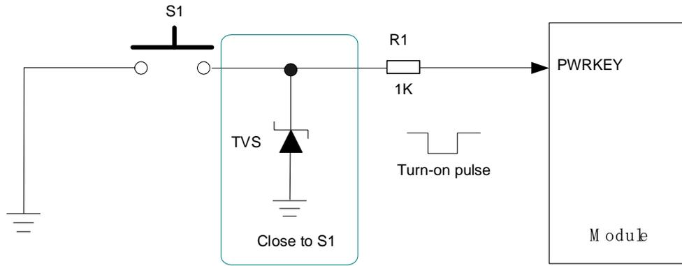
**Figure 8: Turn On the Module Using a Button**
