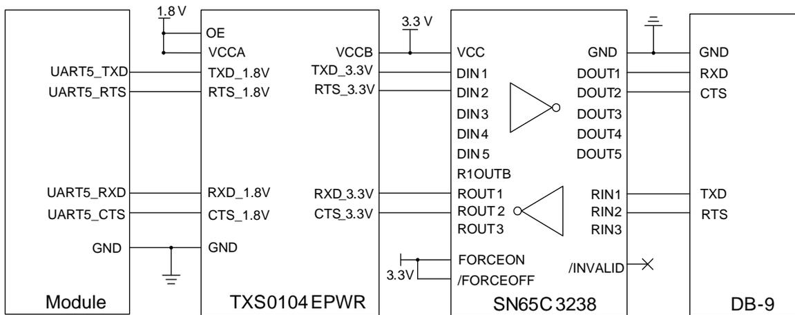
Figure 17: RS-232 Level Matching Circuit (for UART 5)
