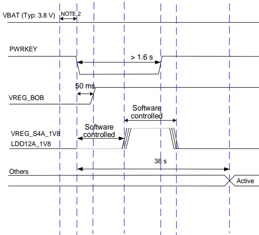
**Figure 10: Power-up Timing**
