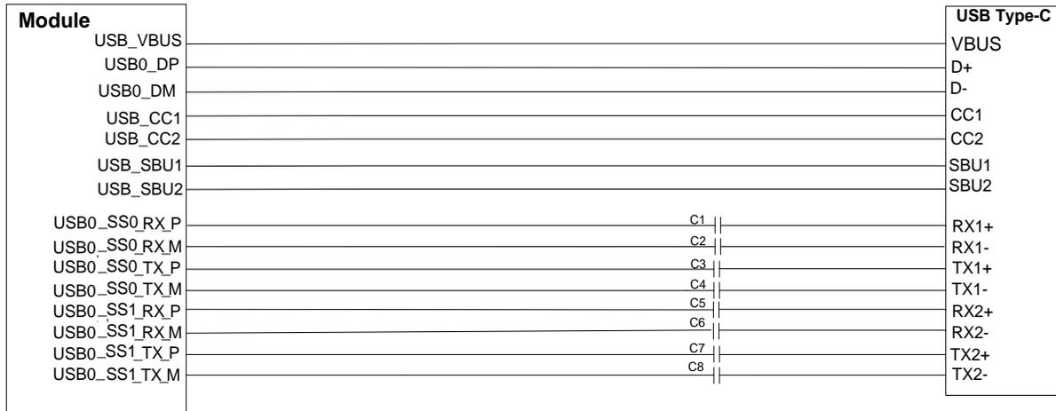
**Figure 14: USB Type-C Interface Reference Design**
