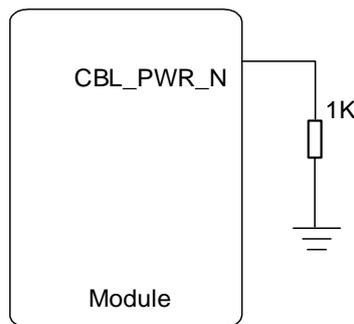
**Figure 9: Reference Circuit of Automatic Turn-on**
