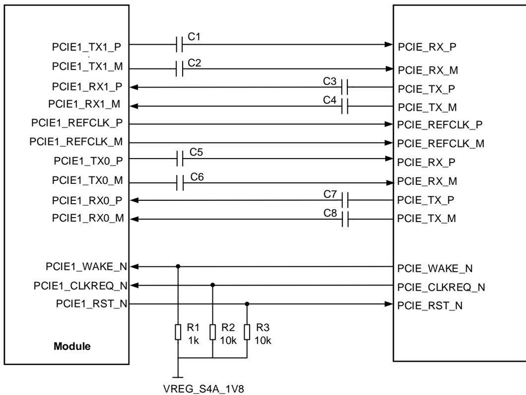
**Figure 19: Reference Design of PCIe1 Interfaces**
