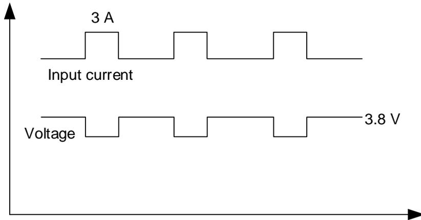
**Figure 5: Voltage Drop Sample**
