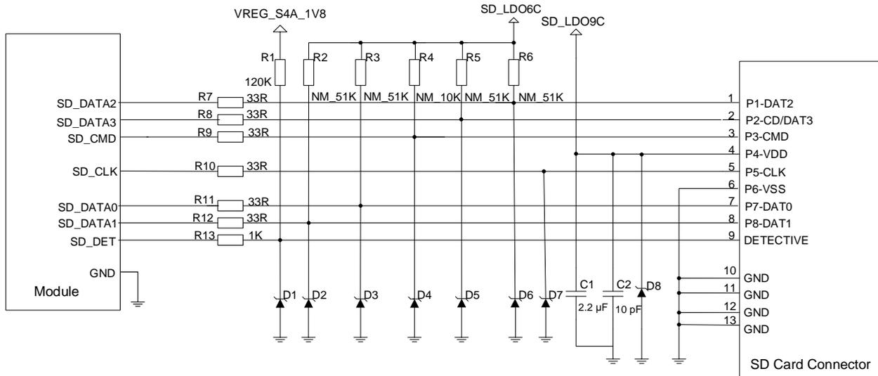
Figure 18: Reference Circuit for SD Card Interface
