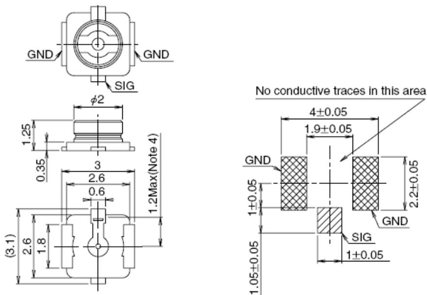
**Figure 33: Dimensions of the Receptacle (Unit: mm)**
