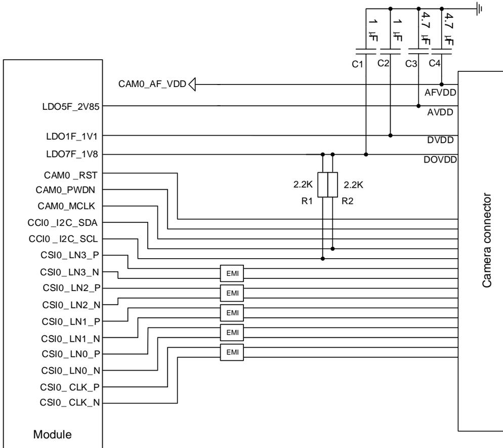
Figure 24: Reference Design for Camera0 Application
