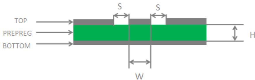
**Figure 30: Coplanar Waveguide Design on a 2-layer PCB**
