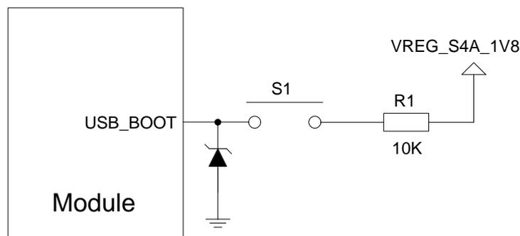
**Figure 27: Reference Design for USB\_BOOT**
