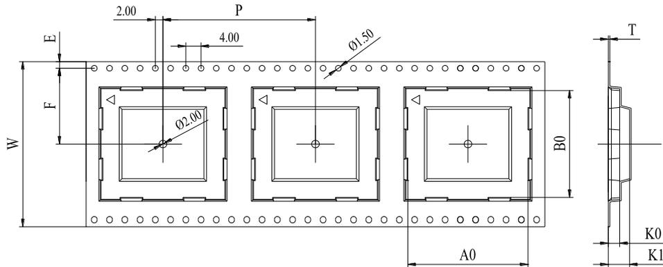
**Figure 41: Carrier Tape Dimension Drawing**
