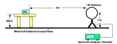
For radiated emissions from 30MHz to 1GHz
