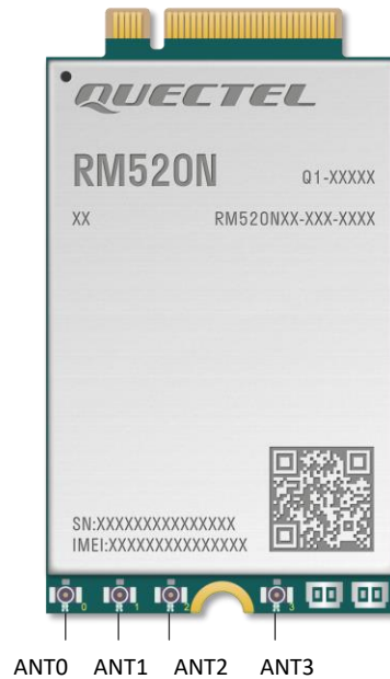
Figure 26: RM520N-GL Antenna Connectors
