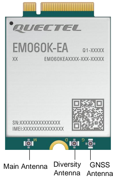
Figure 29: Antenna Connectors on EM060K-EA
