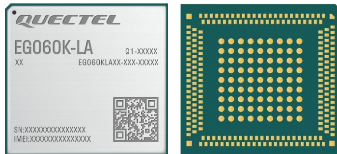
Figure 47: Top and Bottom Views of EG060K-LA
