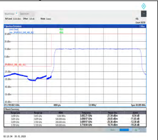
1-N78-3700-3800-30-20-L-3-DFT-PI2BPSK-Outer _Full-50@0-Ant1-1--PASS-see graph
