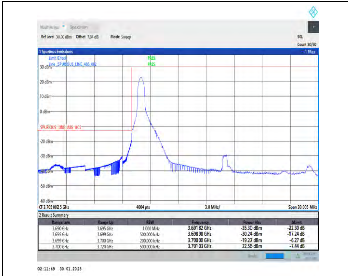
1-N78-3700-3800-30-20-L-1-DFT-PI2BPSK-Edge_1RB _Left-1@0-Ant1-1--PASS-see graph
