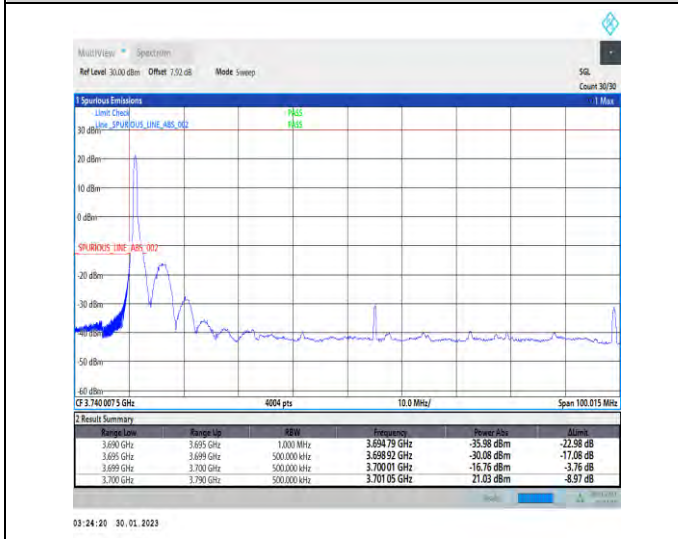
1-N78-3700-3800-30-90-L-4-CP-QPSK-Edge_1RB_Lef t-1@0-Ant1-1--PASS-see graph
