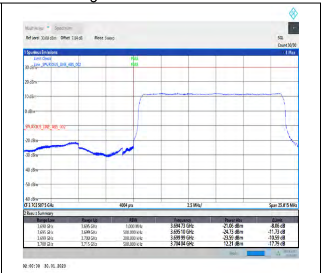
1-N78-3700-3800-30-15-L-3-DFT-PI2BPSK-Outer _Full-36@0-Ant1-1--PASS-see graph
