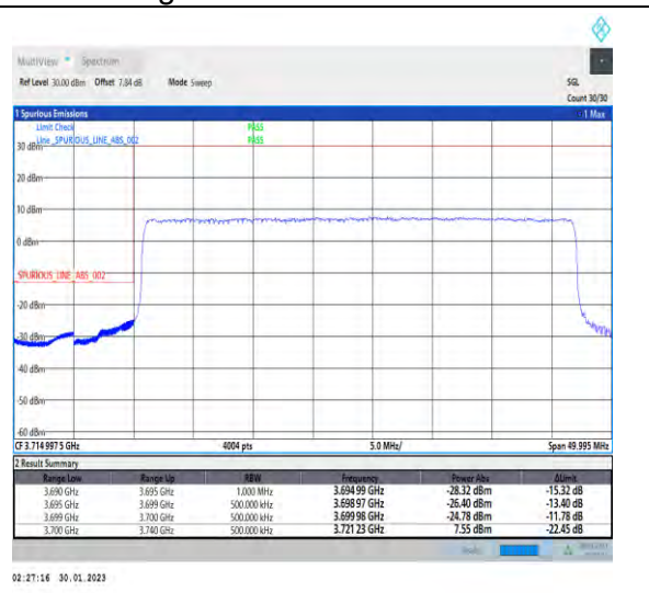
1-N78-3700-3800-30-40-L-3-DFT-PI2BPSK-Outer_Full-100@0-Ant1-1--PASS-see graph
