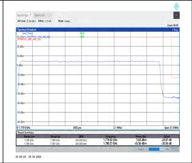
1-N66--15-20-H-3-DFT-PI2BPSK-Outer_Full-100 @0-Ant1-seegraph-PASS-see graph
