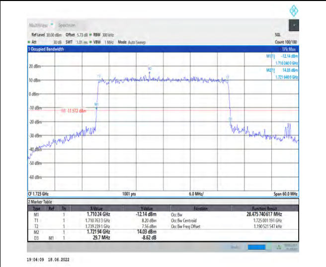
1-N66--15-30-L-4-DFT-64QAM-Outer_Full-160@0-Ant 1-28.476-29.700-≤30-PASS
