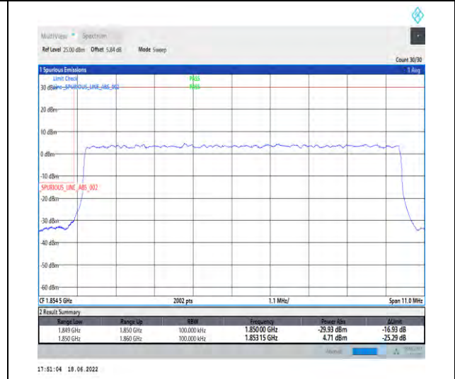
1-N25--15-10-L-3-DFT-PI2BPSK-Outer_Full-50@0 -Ant1-seegraph-PASS-see graph
