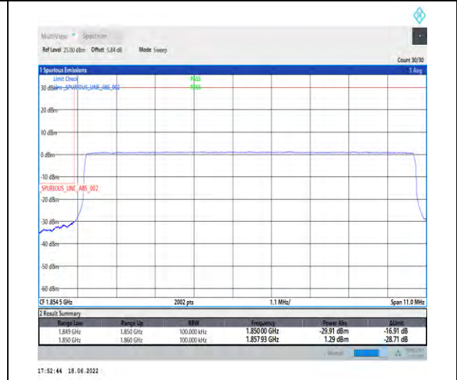
1-N25--15-10-L-6-CP-QPSK-Outer_Full-52@0-Ant1 1-seegraph-PASS-see graph
