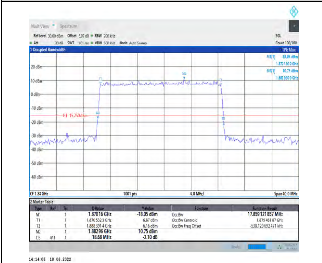
1-N2--15-20-M-5-DFT-256QAM-Outer_Full-100@0-A Ant1-17.859-18.680- \leq 20 -PASS
