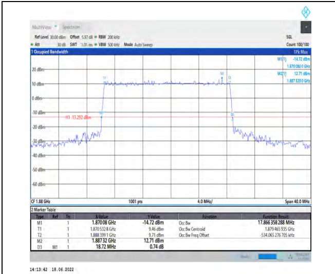
1-N2--15-20-M-3-DFT-16QAM-Outer_Full-100@0-A nt1-17.866-18.720- \leq 20 -PASS
