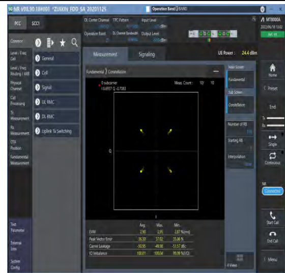
1-N25--15-40-M-2-DFT-QPSK-Outer_Full-216@0-A nt1-see graph-PASS
