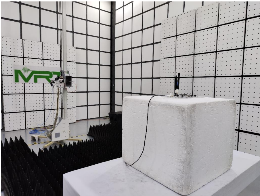
Description: Transmitter Spurious Emissions Test Setup (1GHz ~ 18GHz) For Cellular
