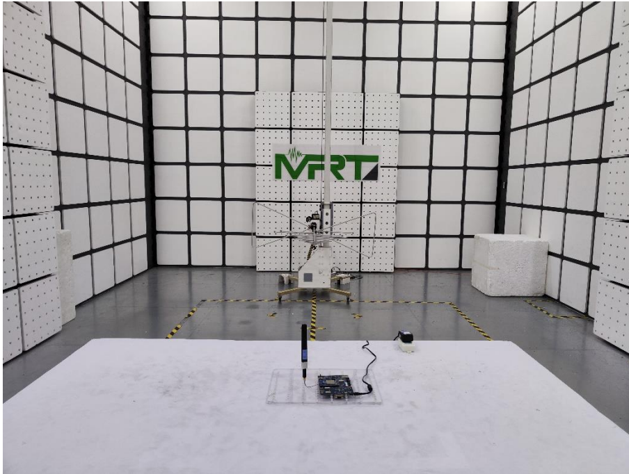
Description: Transmitter Spurious Emissions Test Setup (1GHz ~ 18GHz) For Cellular
