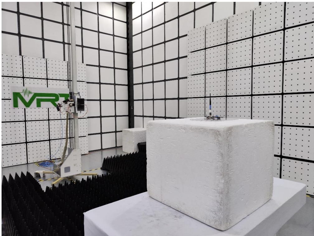
Description: Radiated Spurious Emission Test Setup for above 1GHz For Bluetooth-BR/EDR
