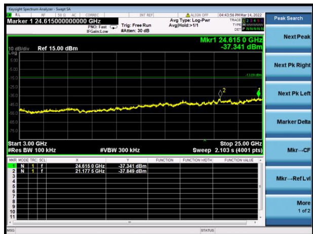
GFSK LOW CHANNEL, SPURIOUS
