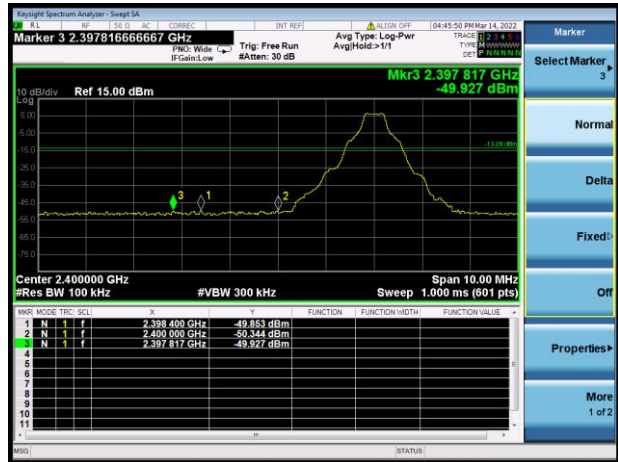
GFSK LOW CHANNEL, BAND EDGE
