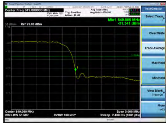
LTE Band 5 QPSK 1.4MHz CH-High 1RB
