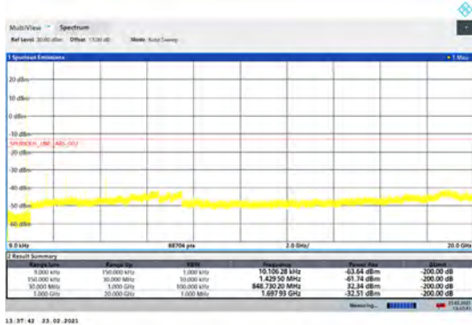
GSM 850 CH-High 9kHz ~ 20GHz
