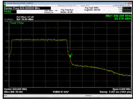
LTE Band 5 16QAM 5MHz CH-High 1RB
