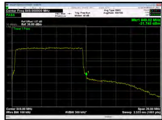
LTE Band 5 16QAM 1.4MHz CH-High 1RB
