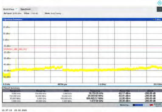
GSM 850 CH-High 9kHz ~ 20GHz
