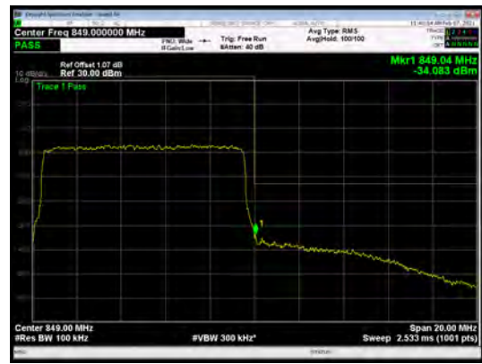
LTE Band 5 16QAM 10MHz CH-High 100%RB
