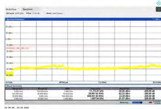
GPRS 850 CH-High 9kHz ~ 20GHz
