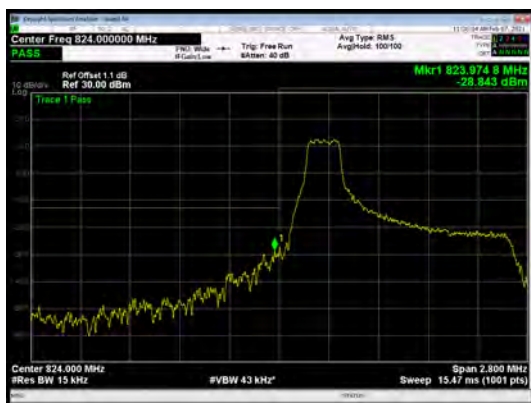
LTE Band 5 16QAM 1.4MHz CH-Low 100%RB
