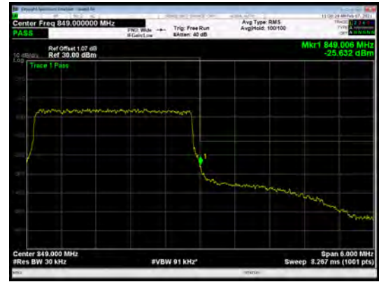
LTE Band 5 QPSK 5MHz CH-High 1RB
