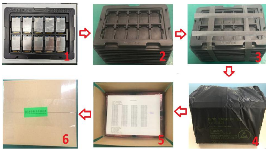
Figure 33: Tray Packaging Procedure
