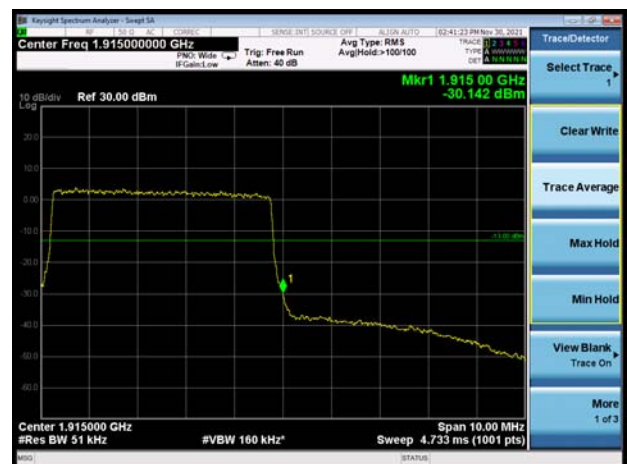
LTE Band 25 5MHz 16QAM 100%RB CH-High
