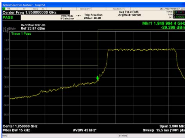
LTE Band 25 3MHz QPSK 1RB CH-Low
