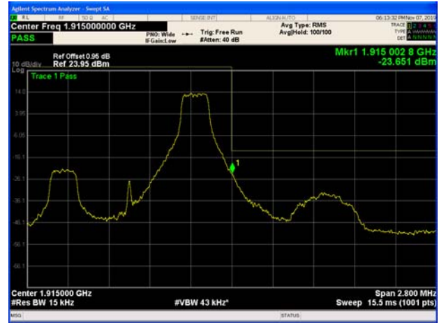
LTE Band 25 1.4MHz QPSK 100%RB CH-High
