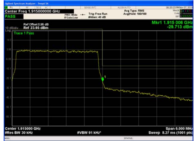
LTE Band 25 5MHz QPSK 1RB CH-High
