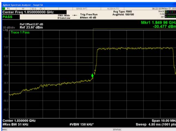
LTE Band 25 5MHz QPSK 100%RB CH-Low
