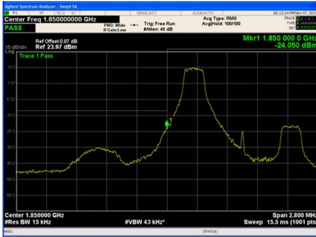
LTE Band 25 1.4MHz QPSK 100%RB CH-Low
