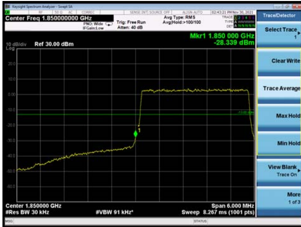
LTE Band 25 5MHz 16QAM 1RB CH-Low
