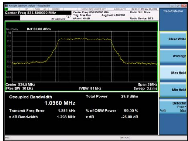
LTE Band 26 16QAM 1.4MHz CH-High
