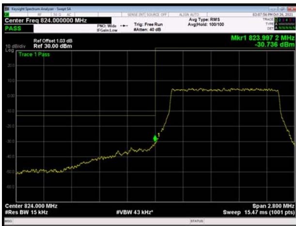
LTE Band 5 1.4MHz QPSK 100%RB CH-Low
