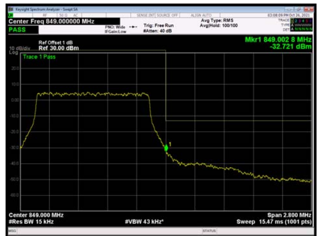
LTE Band 5 1.4MHz QPSK 100%RB CH-High
