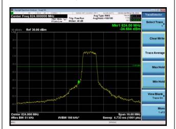
LTE eMTC Band 26 QPSK 3MHz CH-High 100%RB
