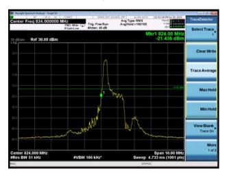
LTE eMTC Band 26 QPSK 1.4MHz CH-High 1RB
