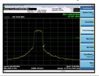
LTE eMTC Band 26 QPSK 3MHz CH-Low 1RB
