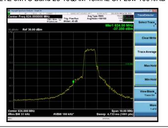
LTE eMTC Band 26 16QAM 15MHz CH-High 100%RB
