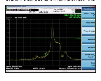
LTE eMTC Band 26 QPSK 15MHz CH-High 1RB
