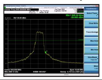
LTE eMTC Band 26 16QAM 5MHz CH-Low 1RB
