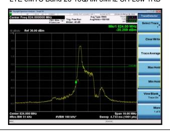
LTE eMTC Band 26 16QAM 5MHz CH-High 1RB
