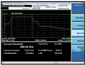
LTE eMTC Band 26 QPSK 5MHz CH-Middle
