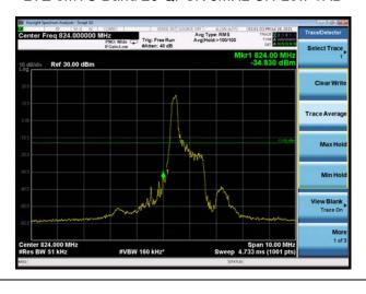
LTE eMTC Band 26 QPSK 3MHz CH-High 1RB
