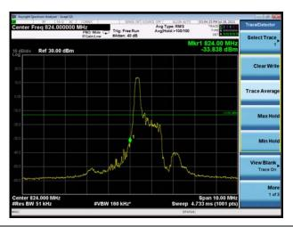
LTE eMTC Band 26 QPSK 5MHz CH-High 1RB
