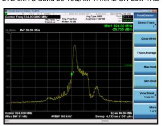
LTE eMTC Band 26 16QAM 1.4MHz CH-High 1RB
